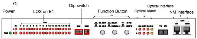
Figure 1: Sketch of the front panel of RC800-480B
